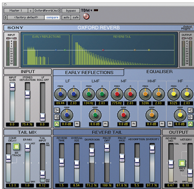
Oxford Reverb control functions are divided into three sections: early reflections, reverb tail processing and mixing/routing.
